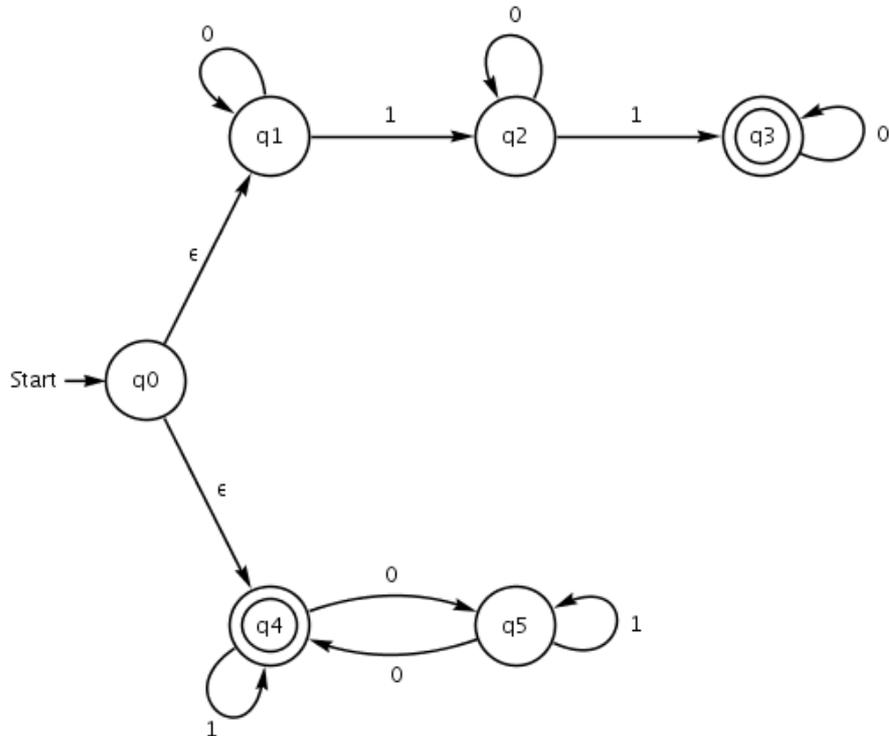
Formal:  $A = \langle \{q_0, q_1, q_2, q_3, q_4, q_5\}, \{\underline{0}, \underline{1}\}, \delta, q_0, \{q_3, q_4\} \rangle$
