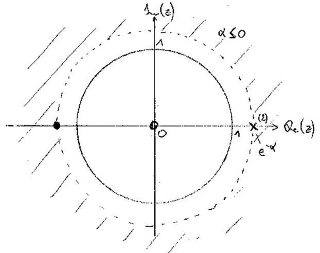
(h)  $x[n] = \delta[n] - \delta[n-10] \rightarrow \frac{z}{z-1} - z^{-10} \frac{z}{z-1} = \frac{z-z^{-9}}{z-1} = \frac{z^{10}-1}{z^9(z-1)}$
